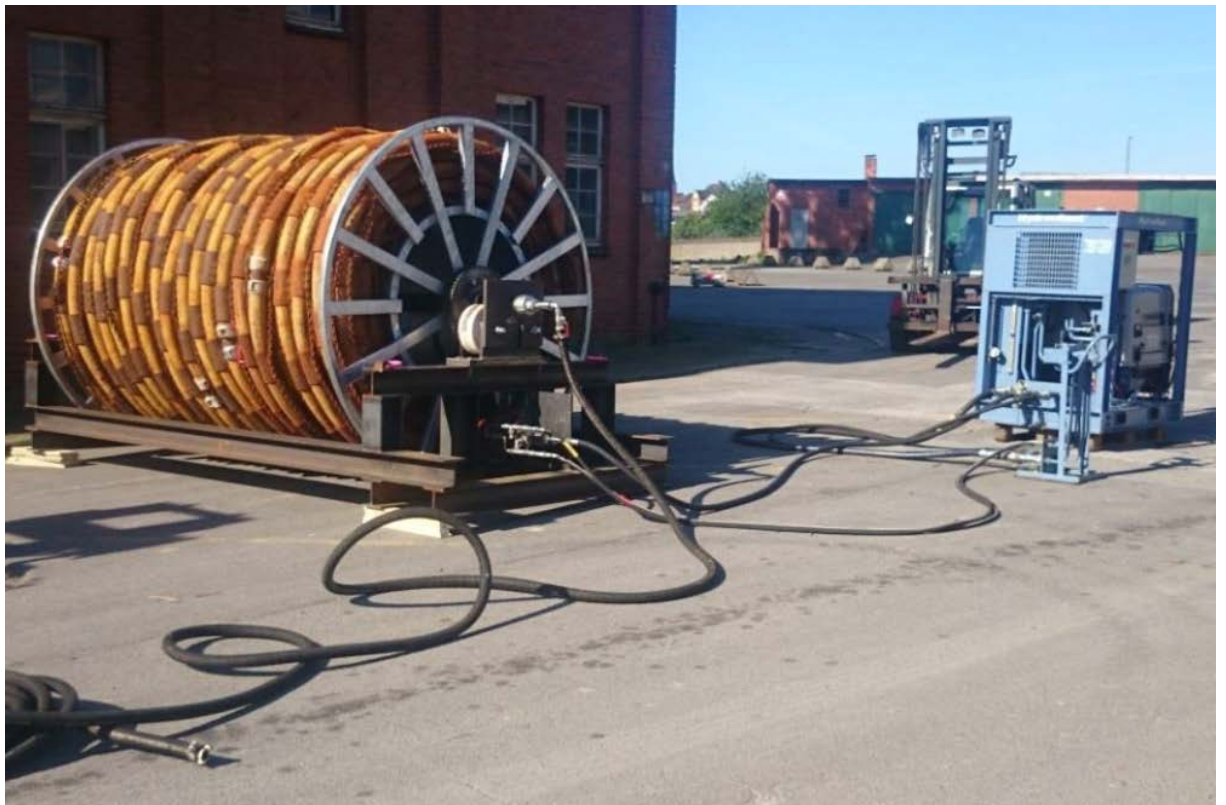
Figure 11.5 : Hose stored on winch
