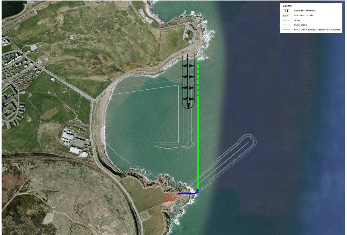
Figure 11.4: Indicative bubble screen position during blasting, connected to the partially constructed breakwater
