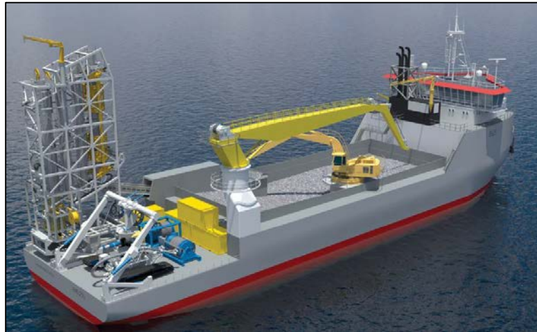
Figure 21 – Marine discharge vessel for rock and bedding material layers
