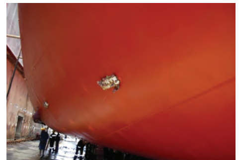
Research vessel after 31 months in service off West Africa and 5 weeks static in Walvis Bay, before washing
