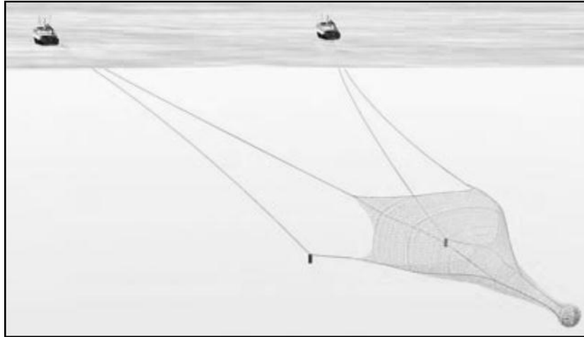
Figure 9.14 Mid Water Pair Trawling
