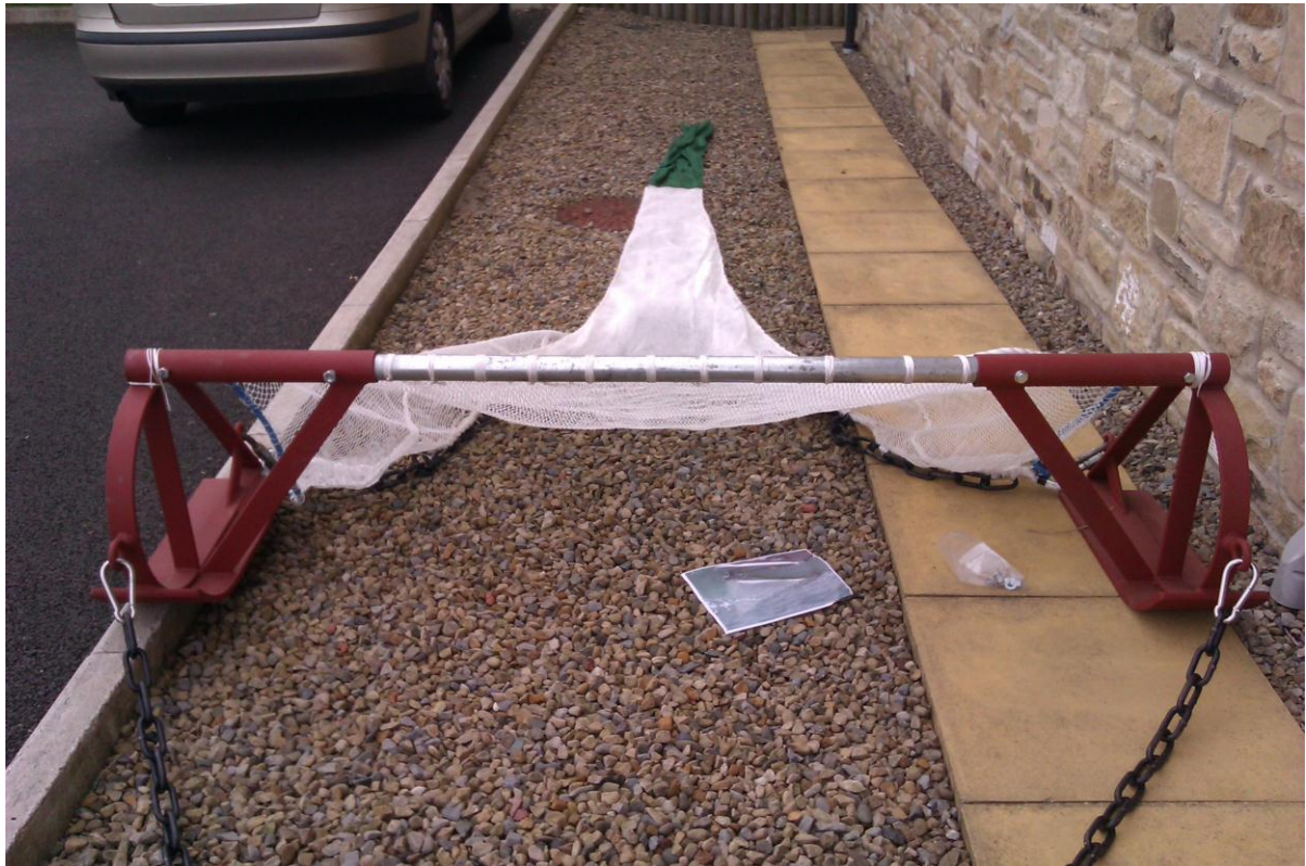
Figure 3: 2 m beam trawl used for the cable route survey
