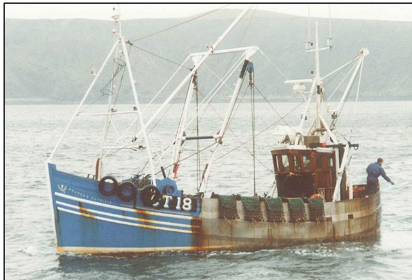
Figure 9.1 Scallop Vessel operating Five Dredges per side (source: BMM)
