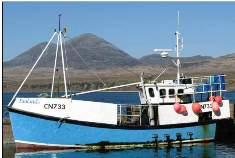
Figure 9.10 Creel Vessel with Vivier Capacity
