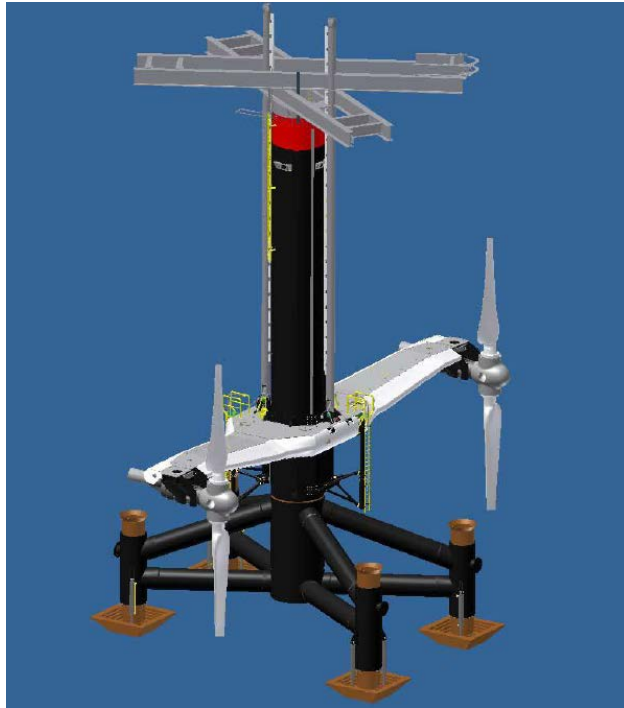
Figure 8 SeaGen S - Example of Quadrapod Foundation
