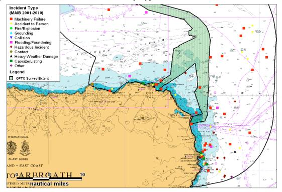
Figure 4.2 Detailed MAIB Incident Locations off Landfall Options by Type within 10nm of the Cable Route
