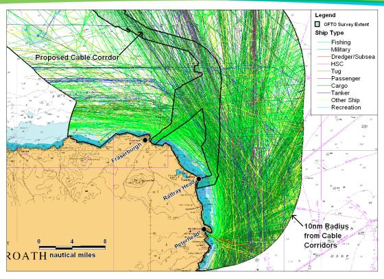
Figure 5.4 Ivero Survey Southern Section of Cable Route (28 Days AIS tracks)
