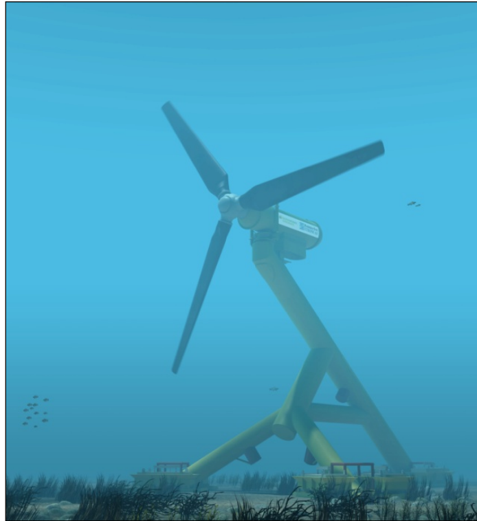
Figure 5 Andritz Hydro Hammerfest 300kW Tidal Turbine
