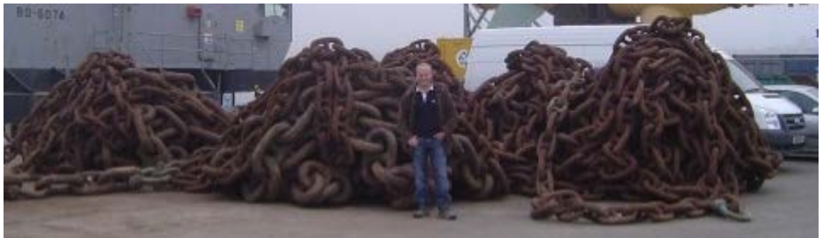
Figure 7 Example chain clumps used by AHH and other contractors in Orkney
