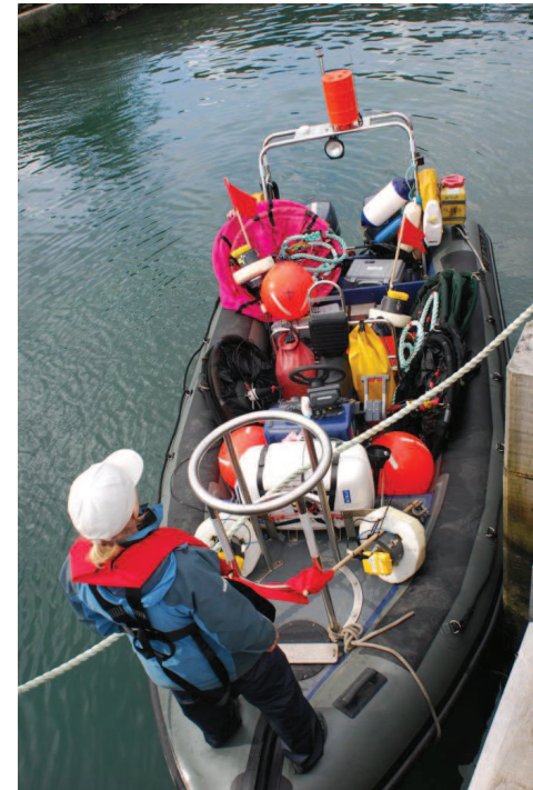
Figure 2. The low-noise RIB Uisge tied up in Port Askaig harbour and used to deploy and retrieve drifters (seen here stowed).
