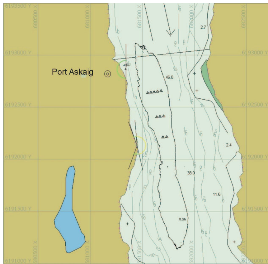
Figure 3. Proposed location for the tidal devices in the Sound of Islay (the 48 m contour shown in black and the proposed turbine sites (black triangles) within the 48 m contour).
