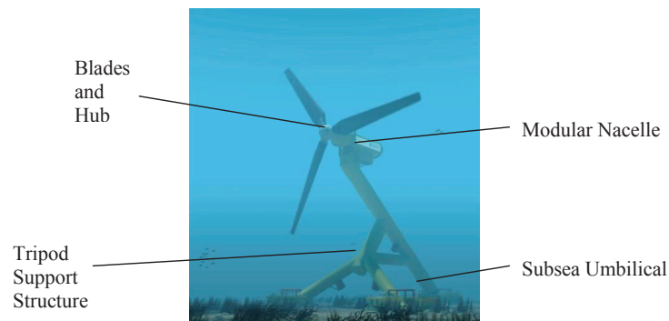
Figure 1. Graphical representation of the 300kW tidal device developed by Hammerfest Strøm, installed in Kvalsund in Finnmark, Norway (SPR, 2008).
