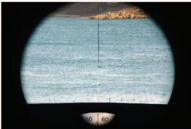
Photograph 6. View through compass binoculars showing compass bearing and vertical graticule.
