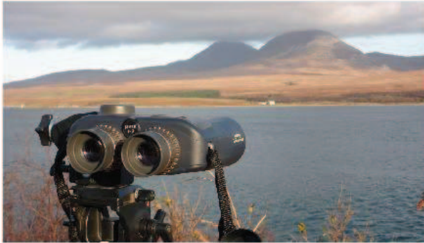
Photograph 5. Compass binoculars mounted level on a tripod. Looking east from cliffs above Port Askaig (at VP 13).
