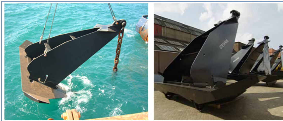
Figure 4.7 Stevpris Mk 5 Drag Embedment Anchor (Image: www.vryhof.com )
