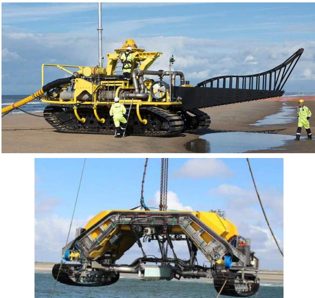
Figure 12 Examples of seabed cable trenching tools (cutting and jetting)
