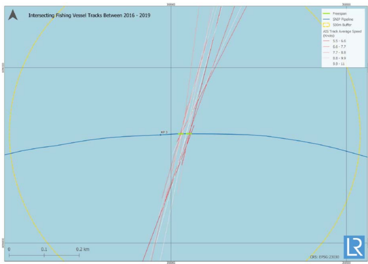
Figure 4-4: Fishing Vessel Track Freespan Interactions (January 1 st 2016 to December 31 st 2018), from Lloyds Registry, 2019)
