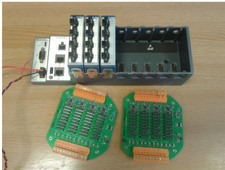
Figure 24: Photograph of the NI Chassis and Etec preamplifier boards purchased for this project.
