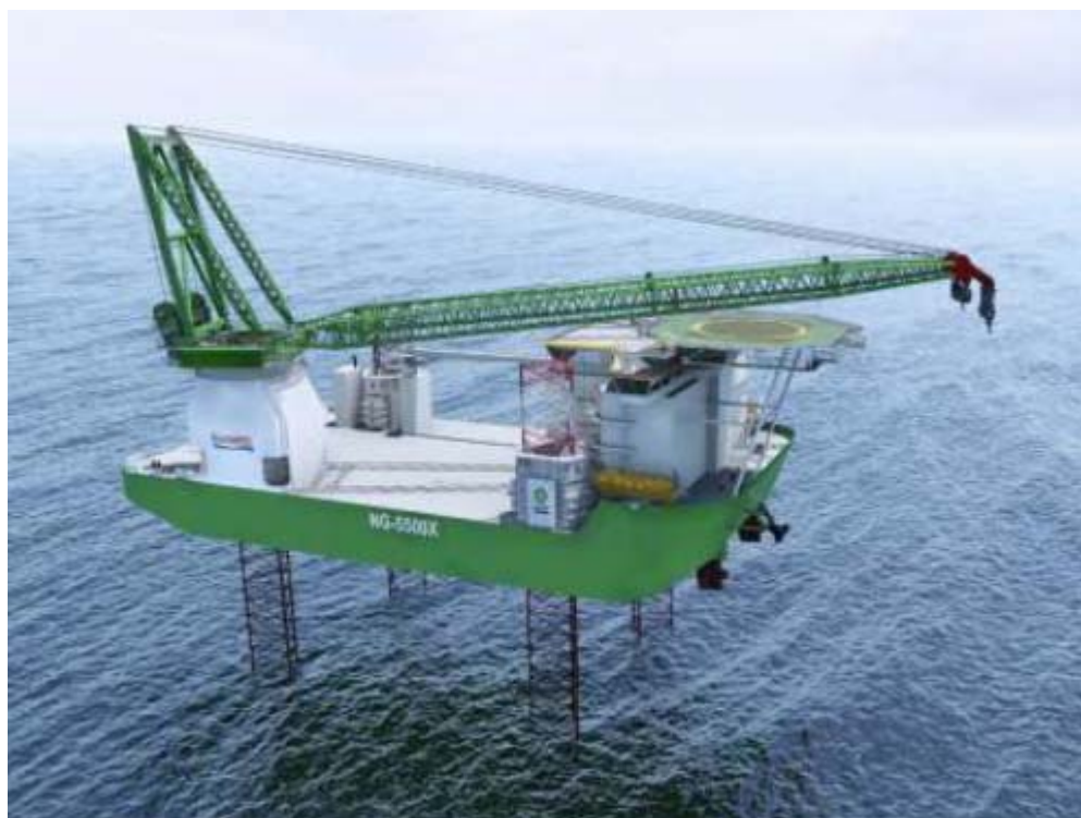
Figure 5-5: Typical Jack-up vessel for piling operations
