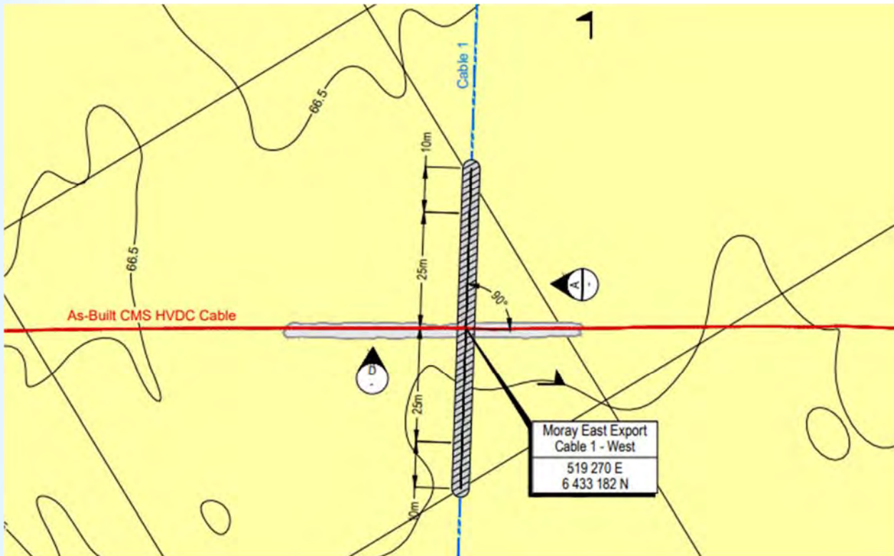
Figure 11-1: Indicative cable crossing arrangement of OEC 1 and SHET HVDC cable.
