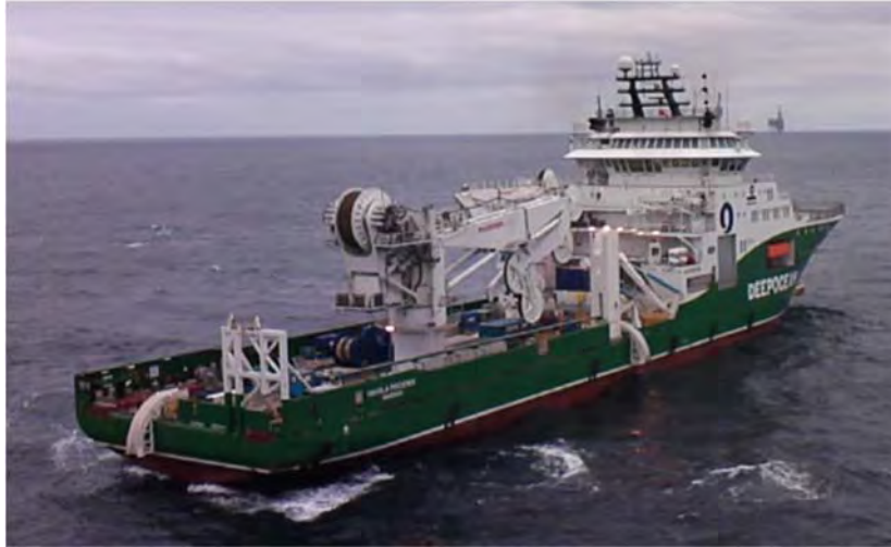
Figure 12-6: Cable Trenching Vessel.
