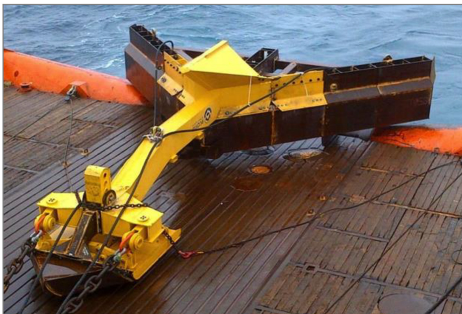
Figure 2-2: Example of a displacement plough
