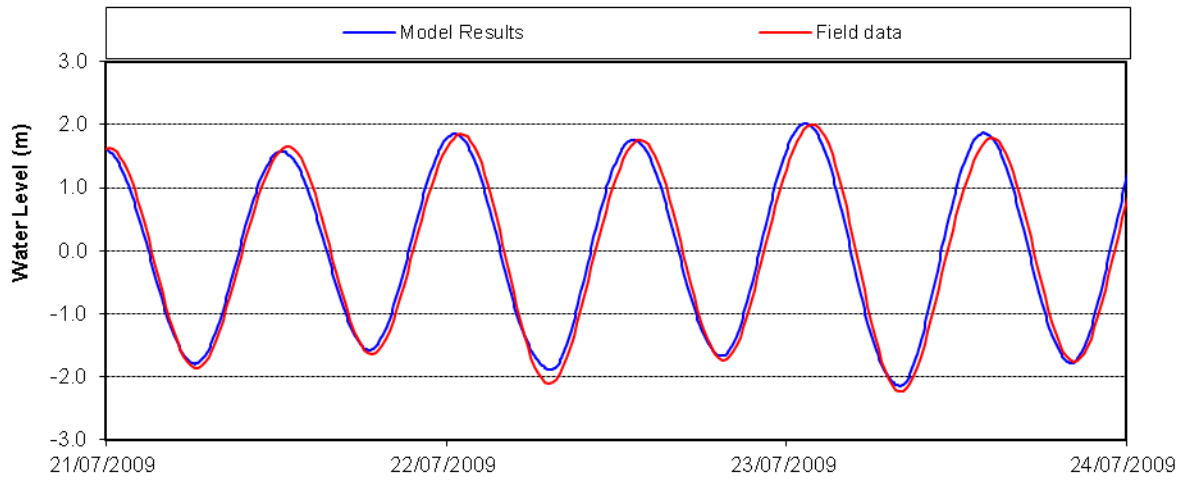
Figure A-29: Model validation for water level at Aberdeen Harbour Admiralty on a spring tide
