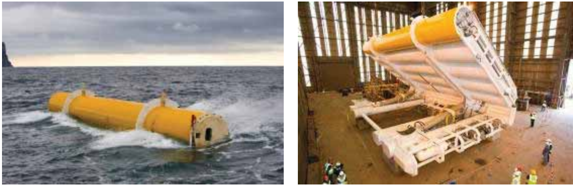
Figure 1.1 (a) & (b) Oyster 1 full scale device in operation / fabrication
