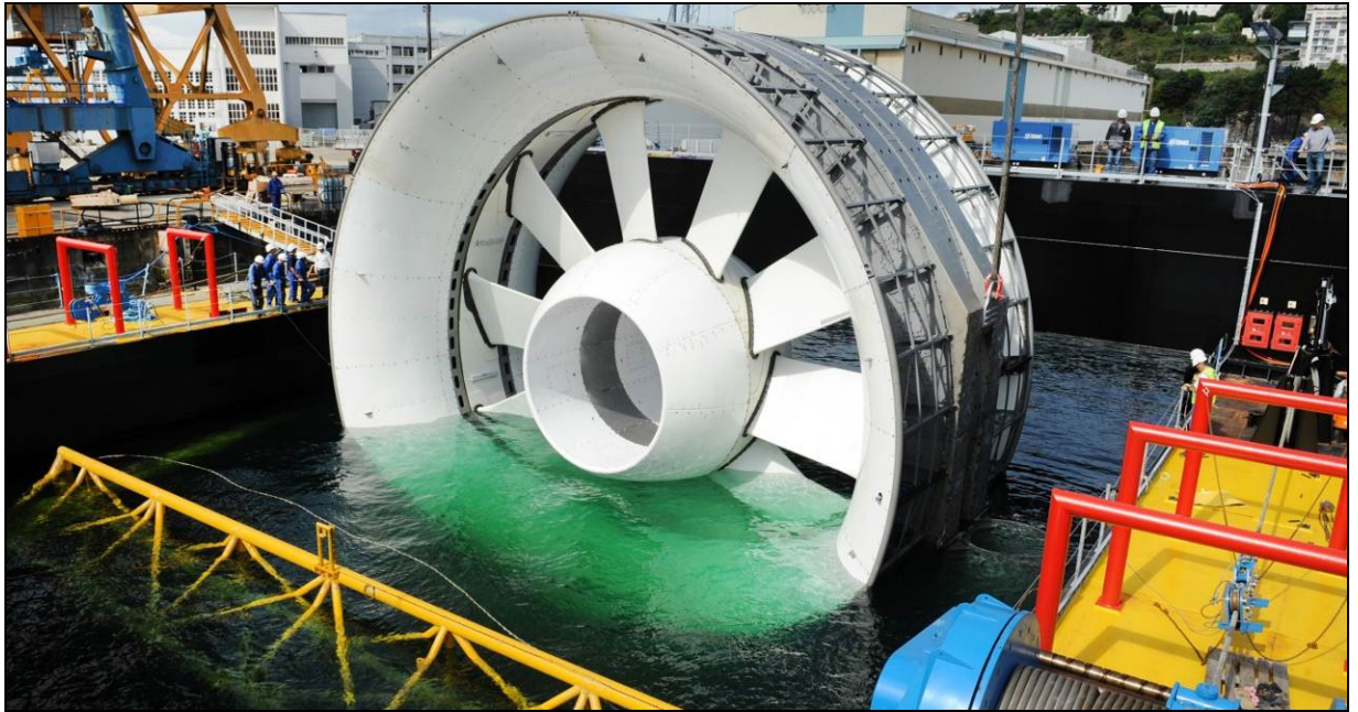
Figure 4.3 - 16m OCT being loaded onto custom-built barge
