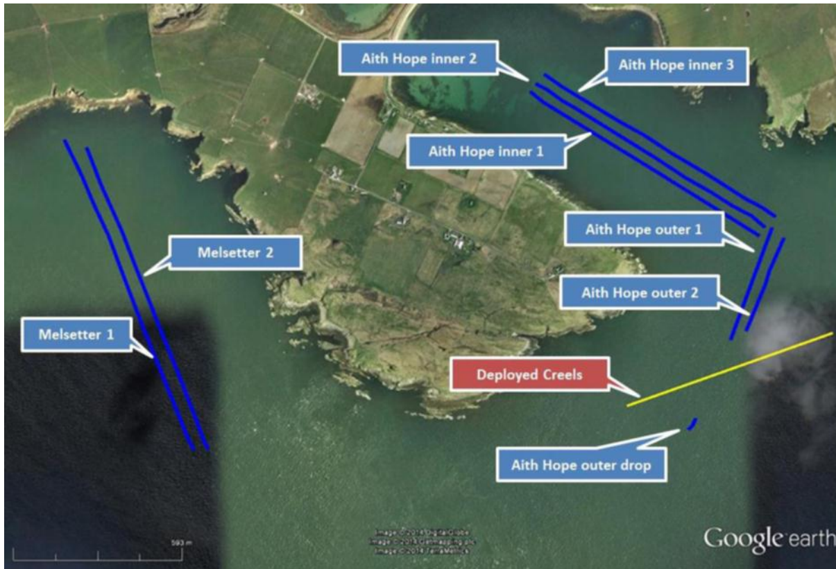
Figure 14: Potential export cable corridors at Aith Hope and Melsetter (aka Moodies Eddy) cable corridor
