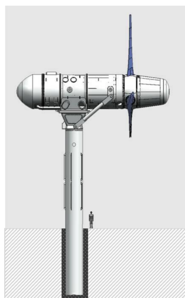
↑ Illustration of single TEC on a monopile structure drilled into the seabed (© Voith Hydro Ocean Current Technologies 2013)
