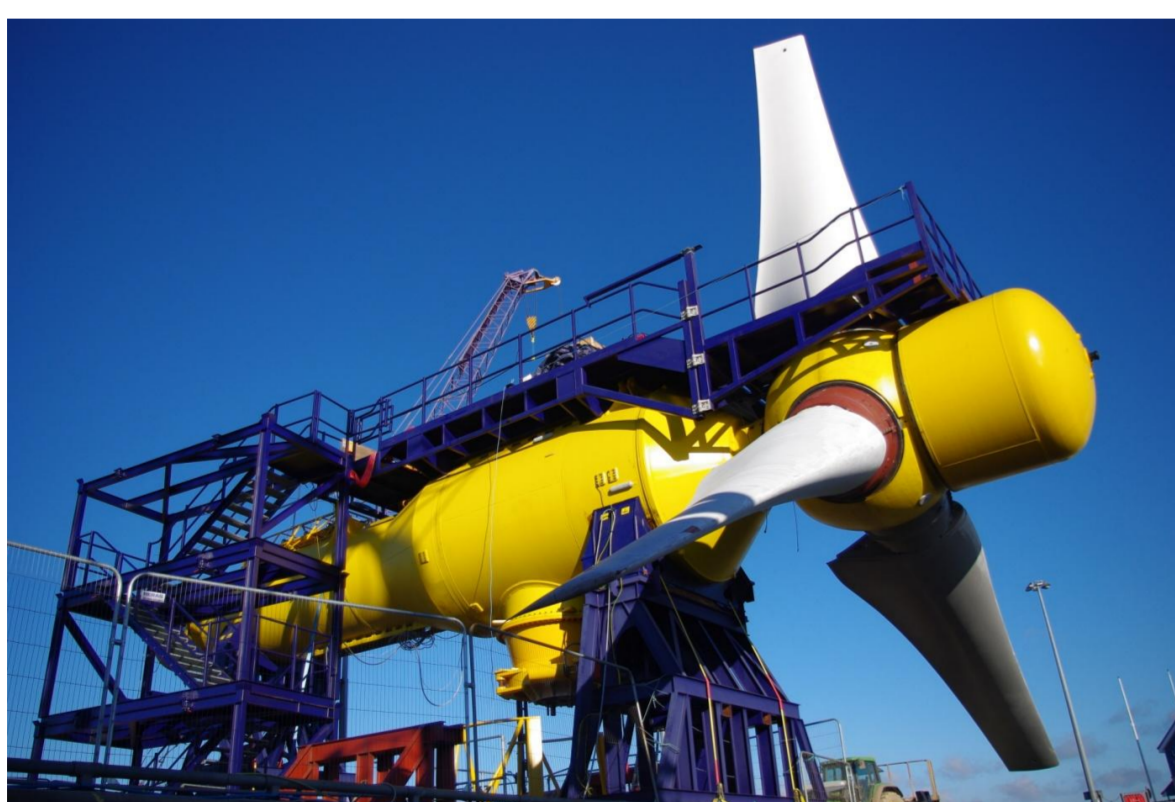
↑ Alstom 3 bladed TEC on quayside at Hatston, Orkney, prior to testing at EMEC (© Alstom 2013)
