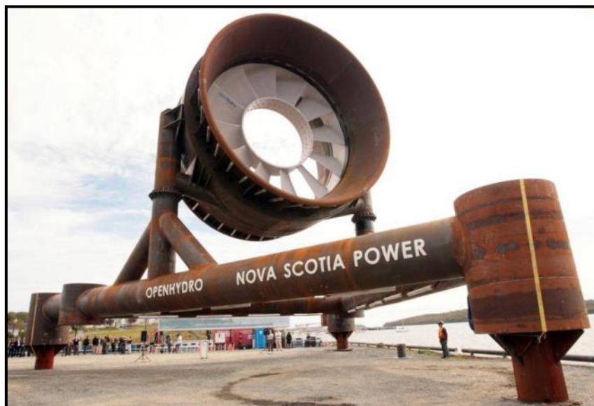
Figure 1.5 Trial assembly of 10m (1MW rated) Open-Centre Turbine & Subsea Base deployed in the Bay of Fundy, Canada – November 2009
