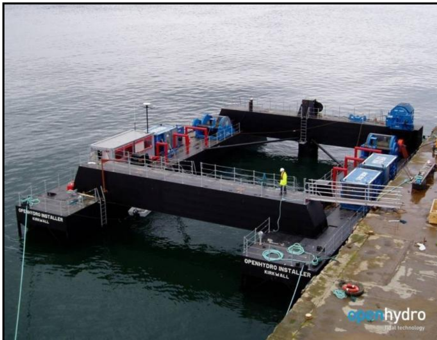
Figure 1.6 OpenHydro Installer turbine installation Barge
