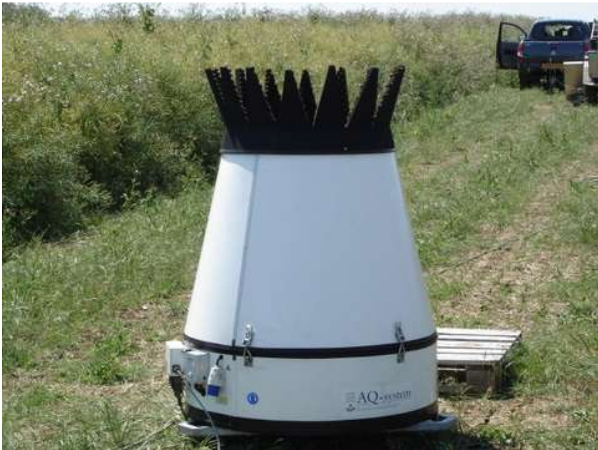
Figure 2.2: AQ500 antenna in standalone setup – most systems now deployed in trailer unit
