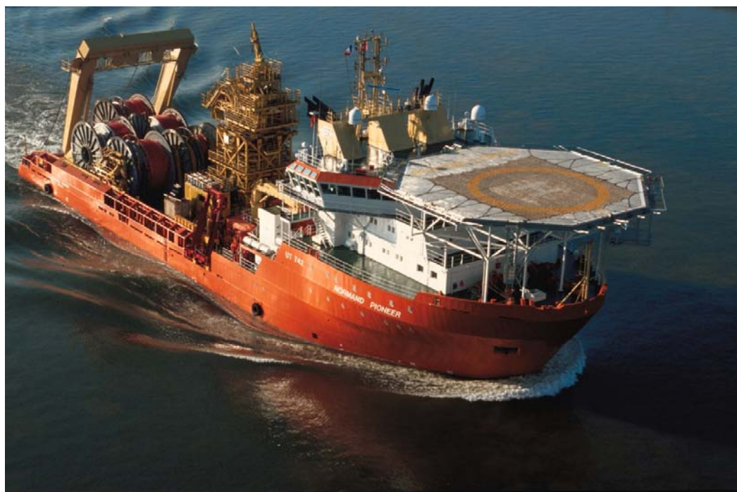
Plate 3.4 Dynamically Positioned Cable Lay Vessel (Courtesy of Technip)
