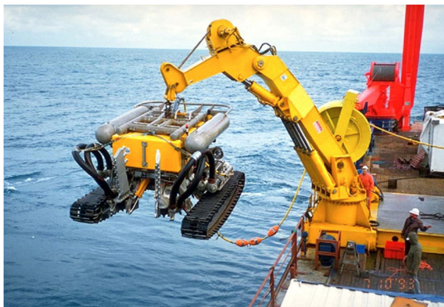
Plate 3.5 ROV Jet Trenching Tool (Courtesy of Technip)
