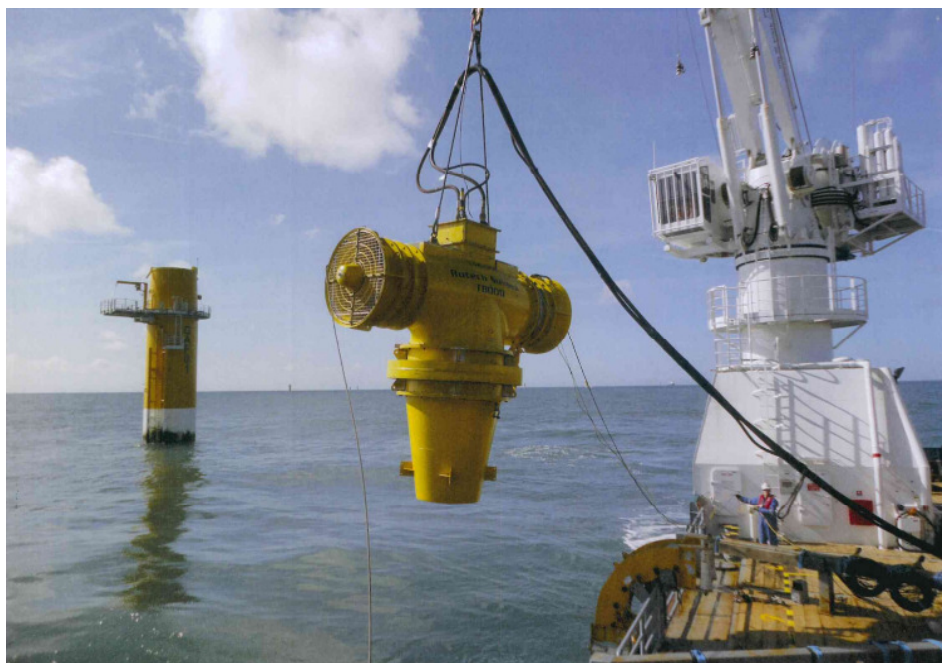
Plate 3.7 Mass Flow Excavation Tool (Courtesy of RoTech)
