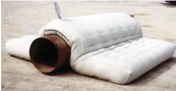
Figure 7.34: Sand-grout Bag Laid over a Test Pipe (Source: BERR)
