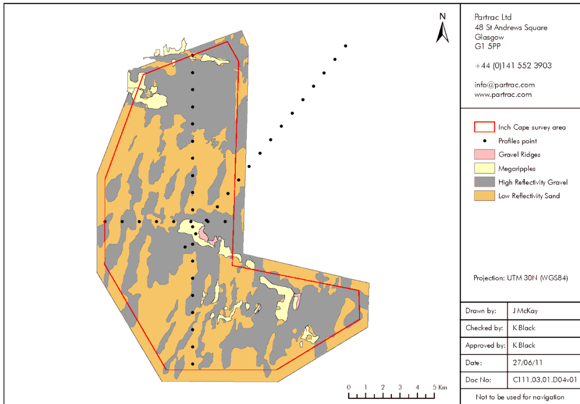
Figure 10A.1.3 Distribution of major sediment types and morphologies across the Inch Cape Development Area. Source Geophysical Survey.
