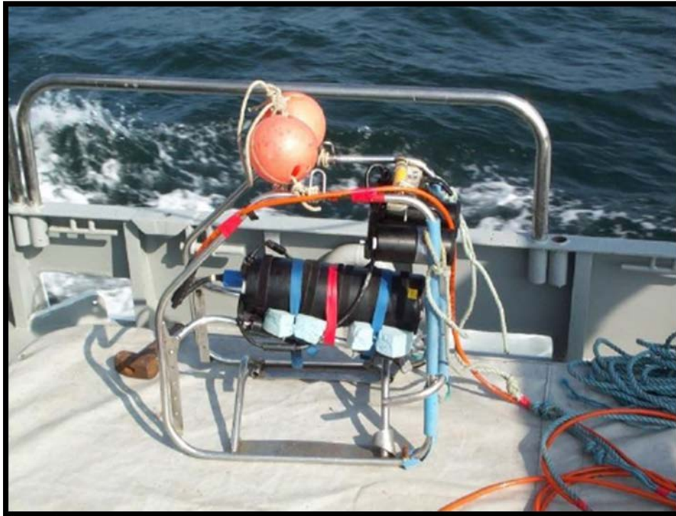
Figure 12A.9 HD Camera within Frame and Housing
