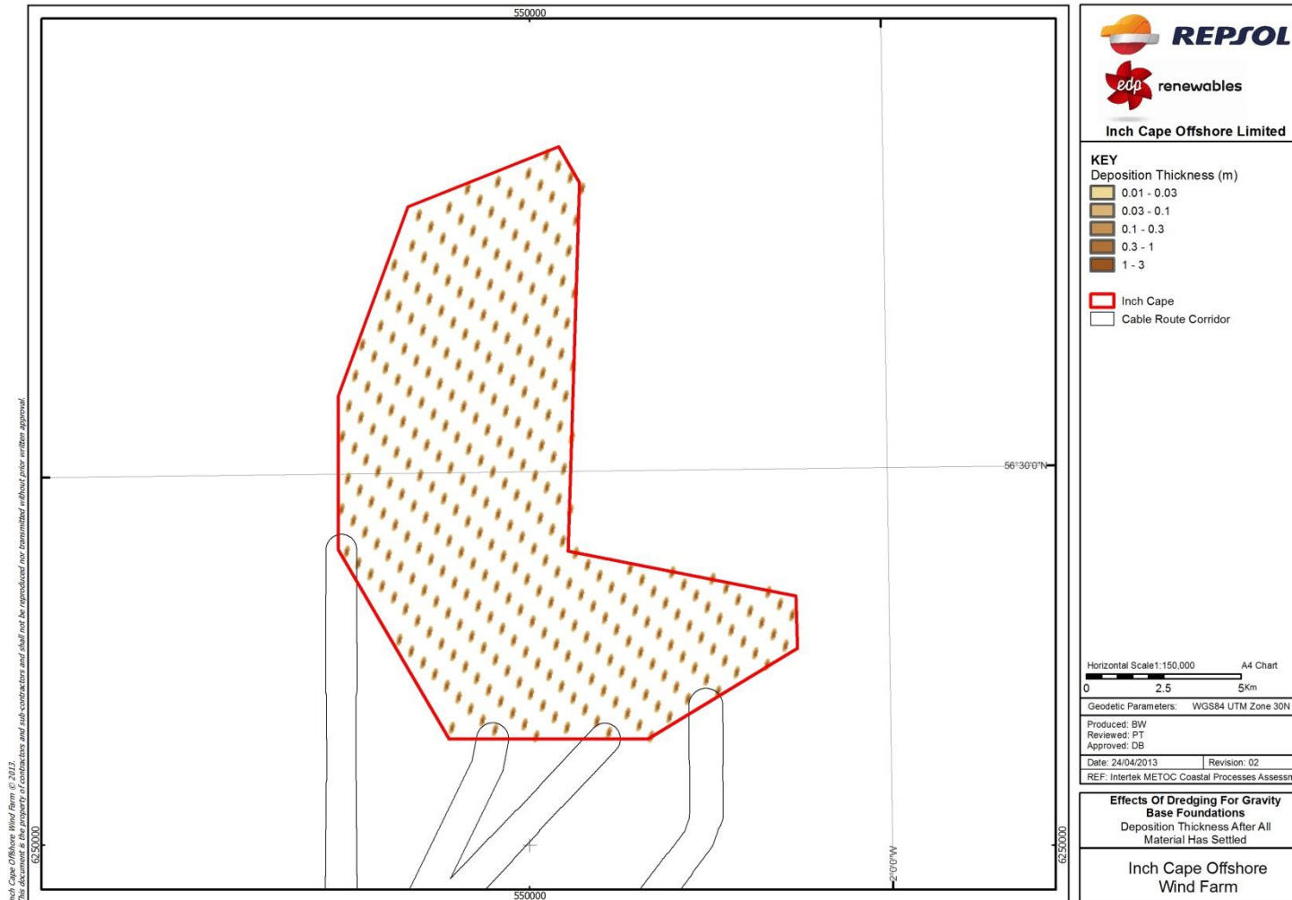
Figure 10.8: Deposition Thickness due to GBS Dredging – after all Material has Settled
