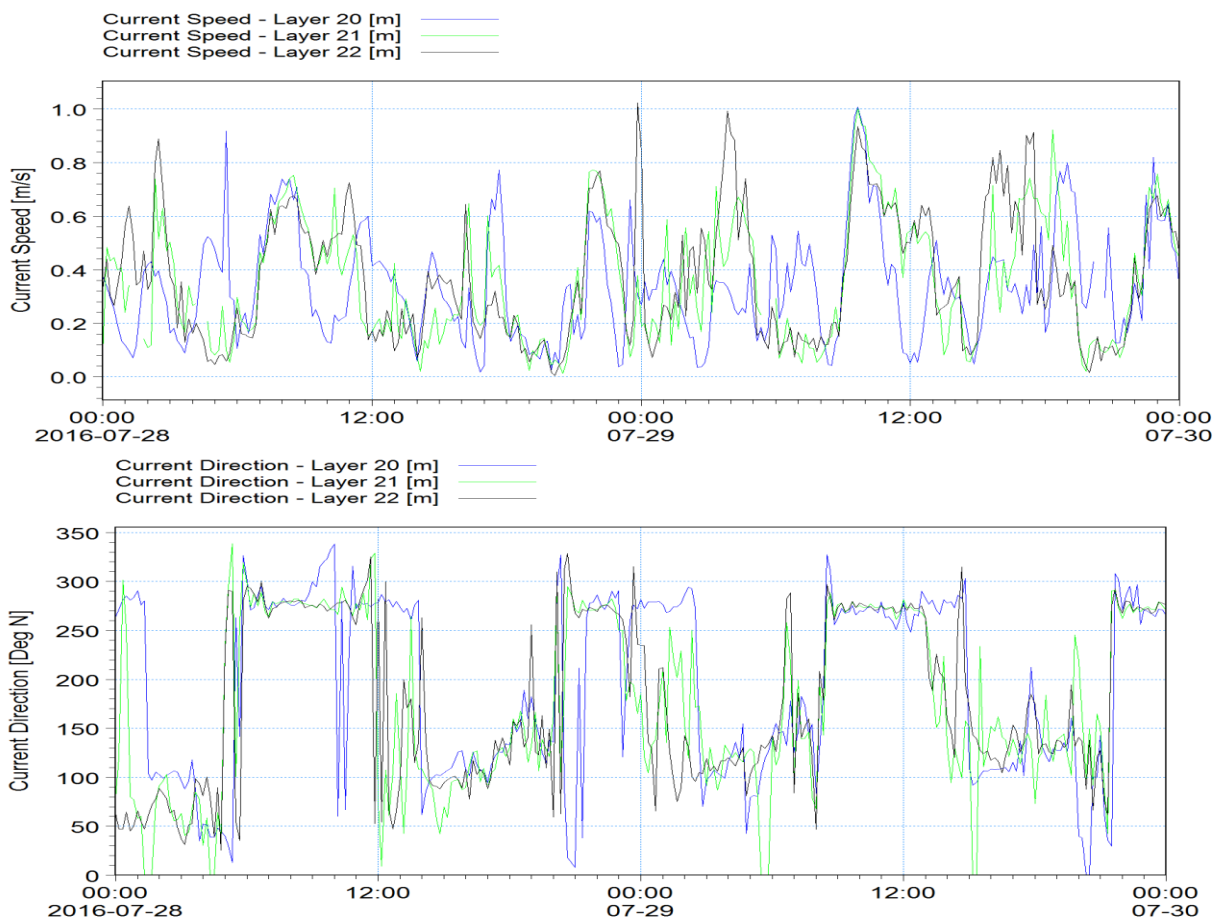
Figure 2.2: Extreme variability of current speeds and directions across three consecutive 0.5m bins – West ADCP.
