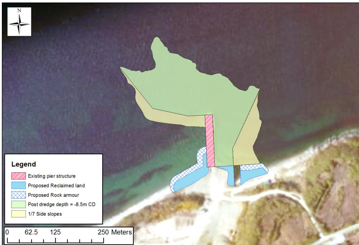
Figure 2.4: Extent of the capital dredging works required as part of the proposed development.
