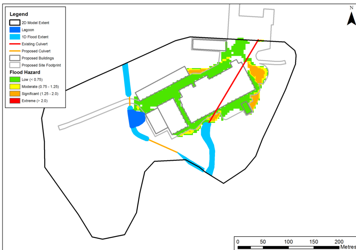
Figure 5-6: Flood hazard (defined by Defra FD2321) for the 0.5% AEP plus climate change scenario with 10% blockage
