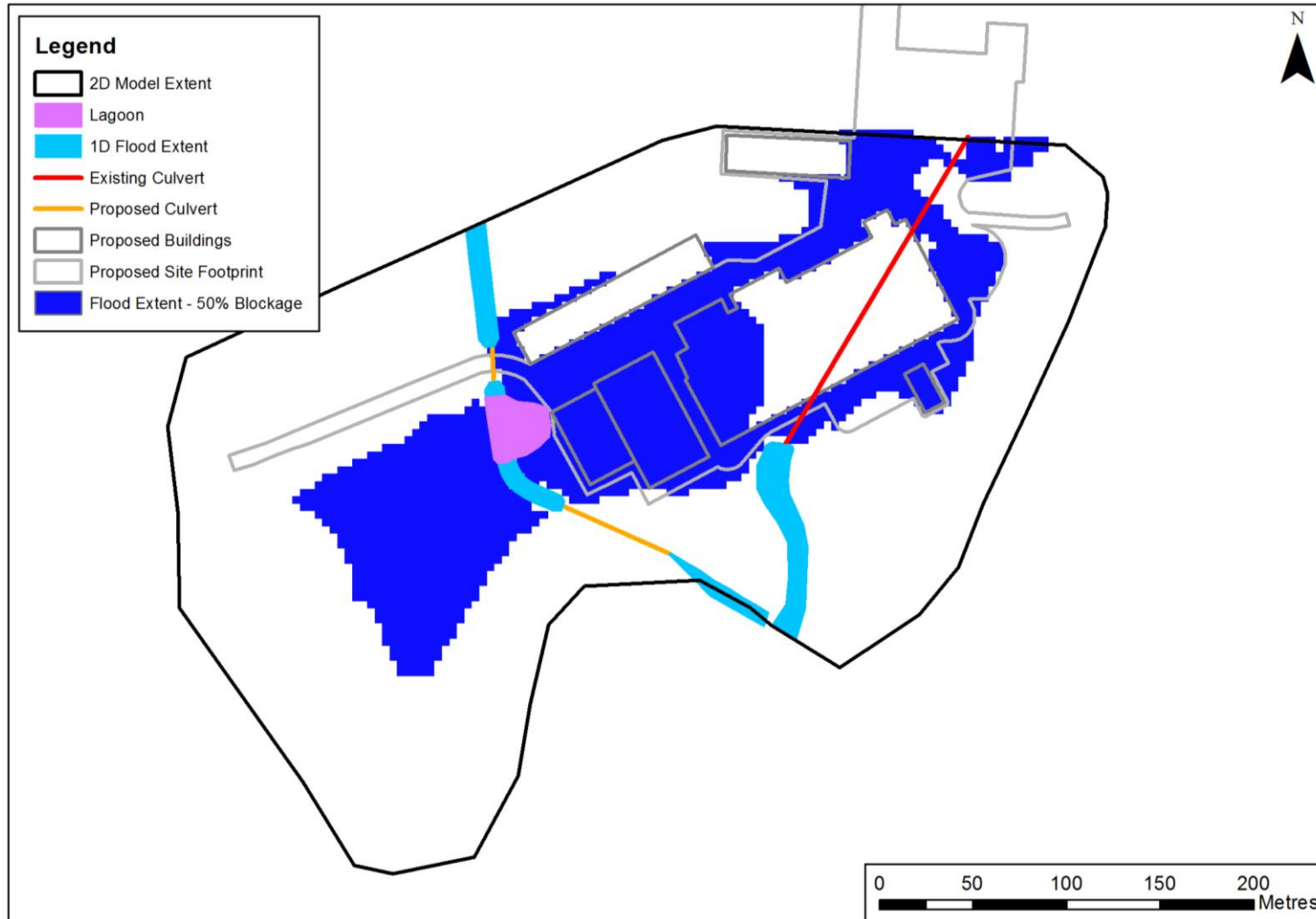
Figure 15: Culvert Blockage to the Proposed 2.5m Culvert - 0.5% AEP plus CC Flood Extent
