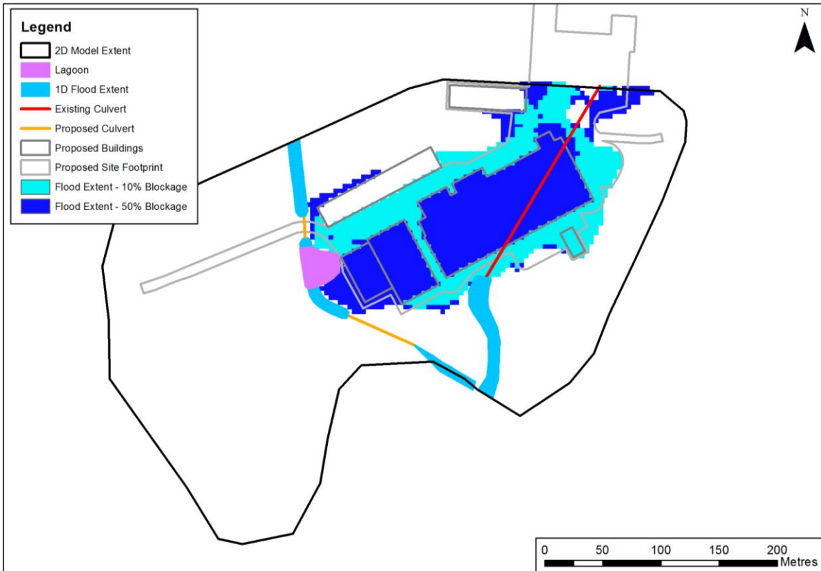
Figure 5-5: Modelled flood extent for Blockage in the Proposed 2.5m Culvert (0.5% AEP plus CC Flood)
