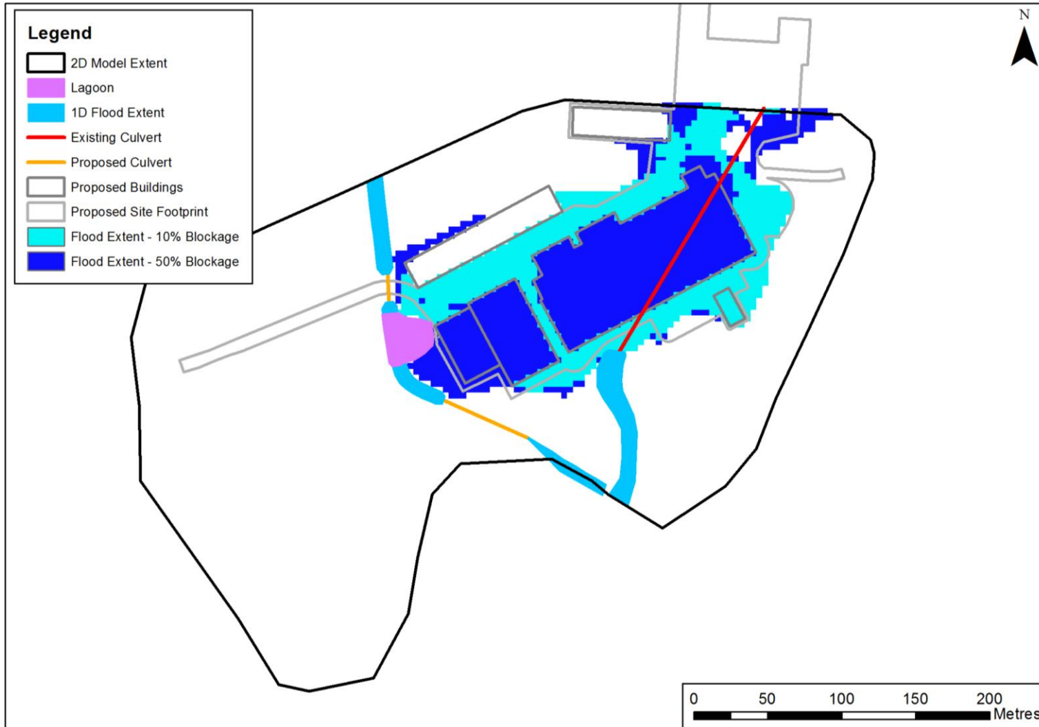
Figure 14: Culvert Blockage to the Proposed 2.5m Culvert - 0.5% AEP plus CC Flood Extent
