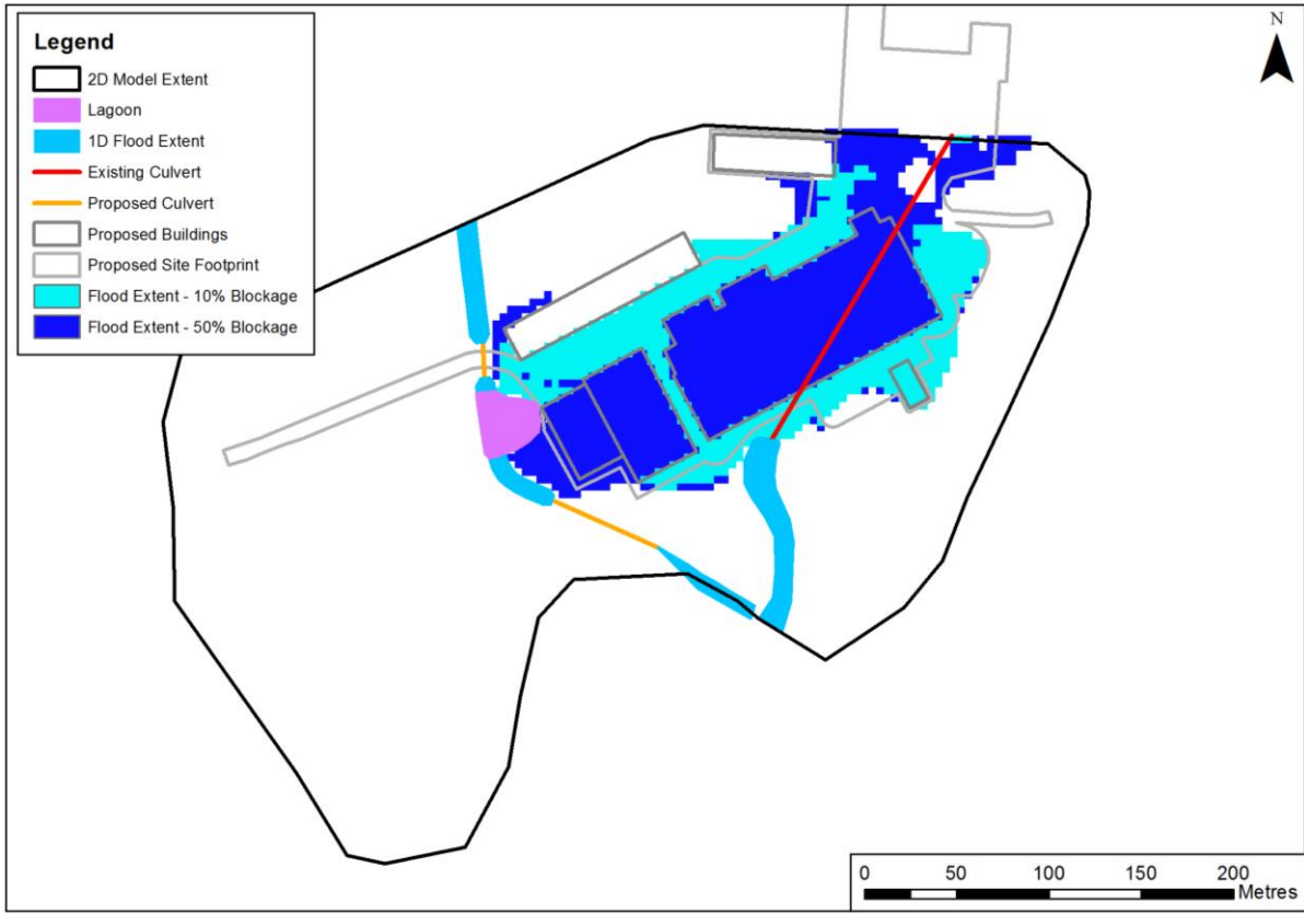
Figure 5-4: Modelled flood extent for Blockage in the Existing Culvert (0.5% AEP plus CC Flood)
