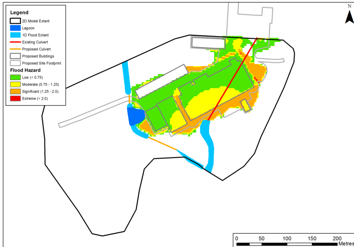
Figure 5-7: Flood hazard (defined by Defra FD2321) for the 0.5% AEP plus climate change scenario with 50% blockage
