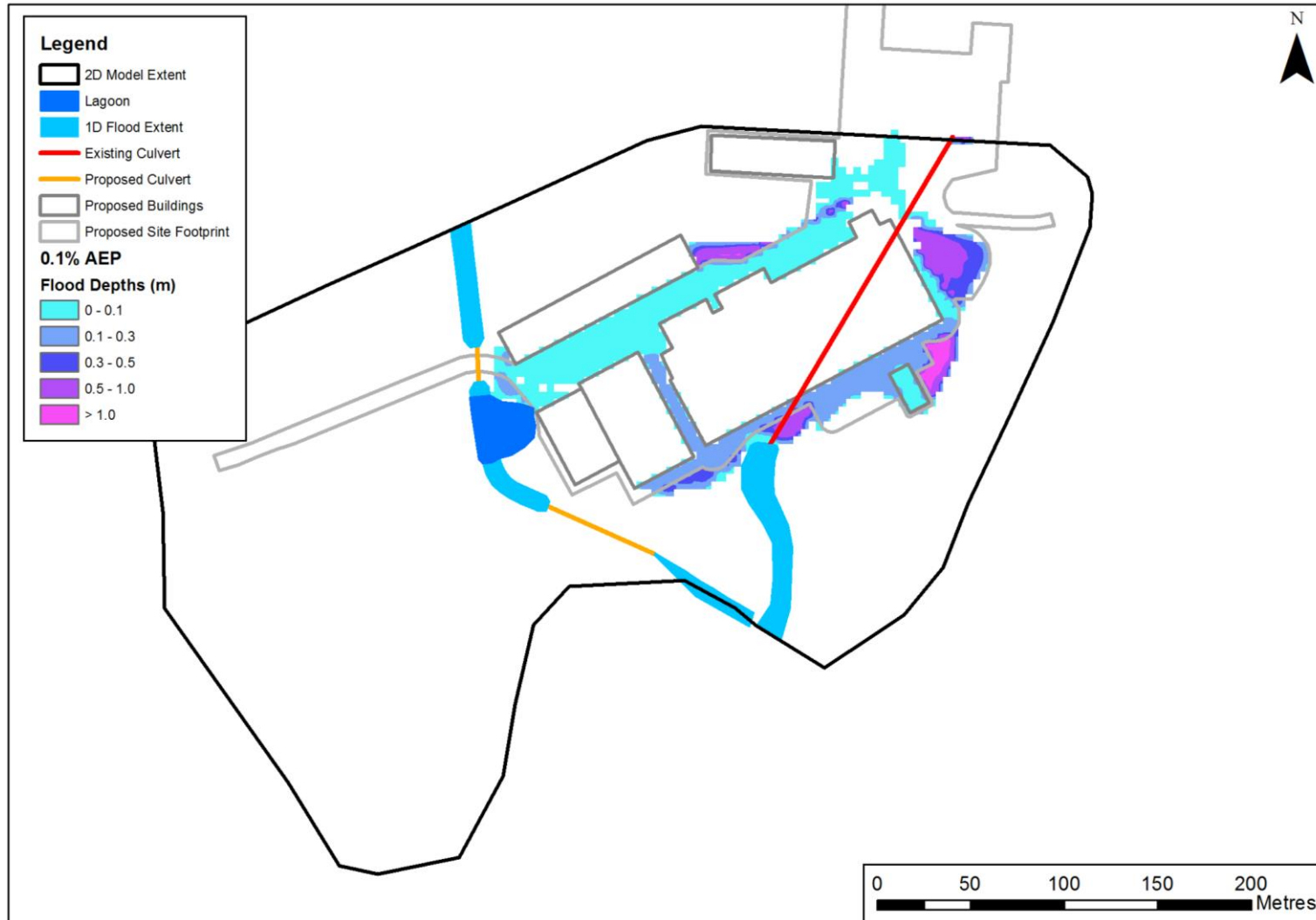
Figure 11: Design Option 0.1% AEP Fluvial Flood Extent
