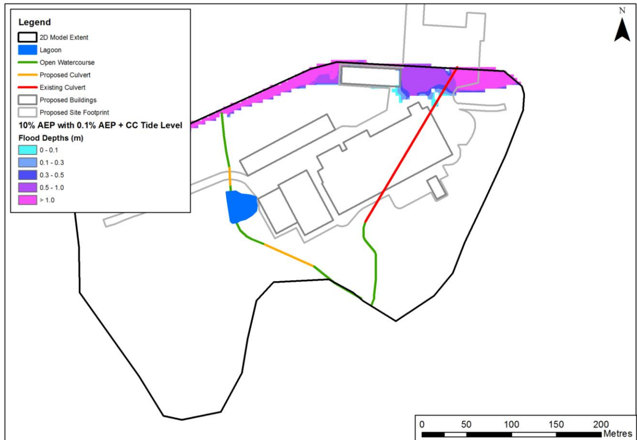
Figure 5-3: Design Option 0.1% AEP Tidal and 10% AEP Fluvial Flood Extent
