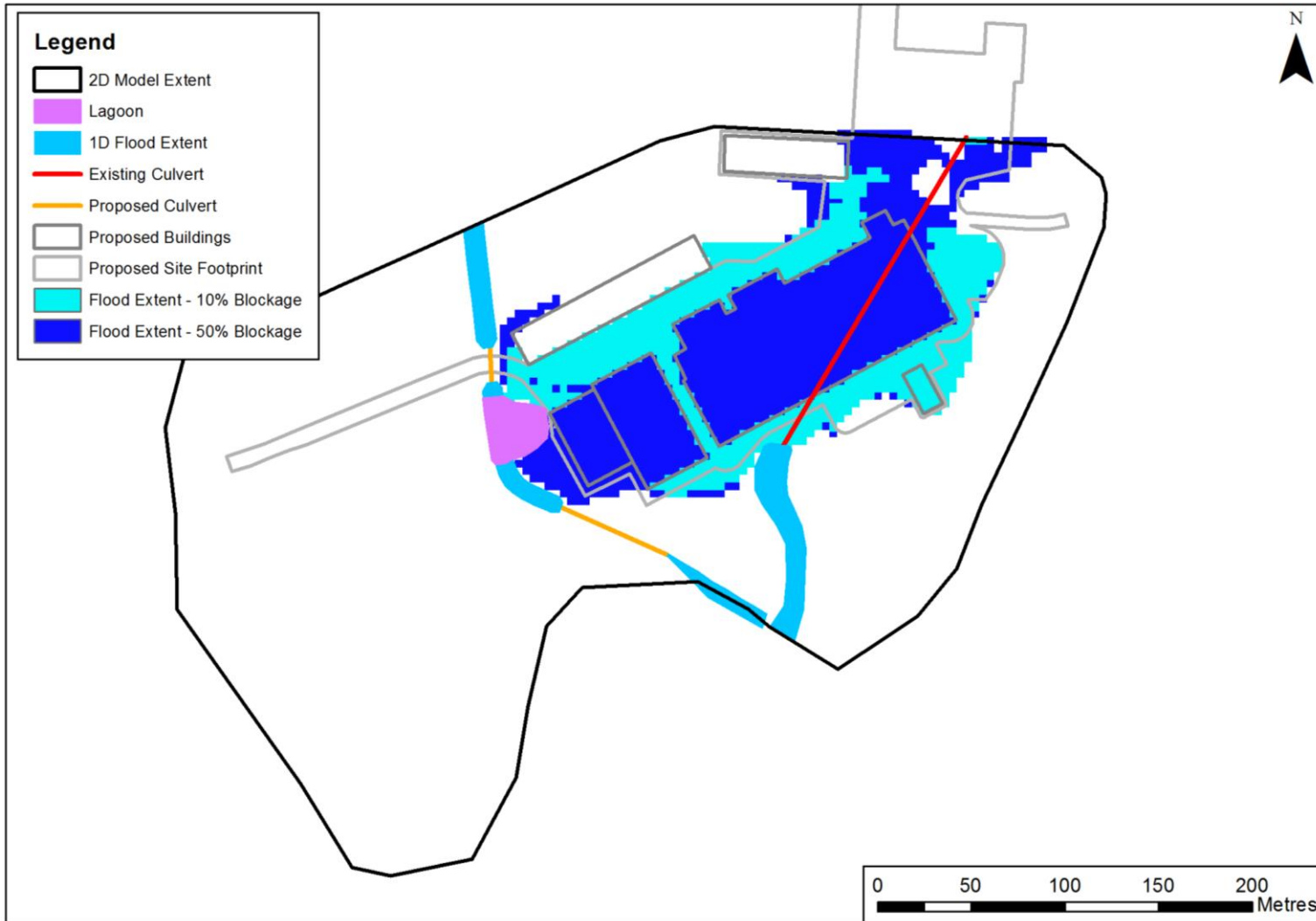
Figure 13: Culvert Blockage to the Existing Culvert - 0.5% AEP plus CC Flood Extent
