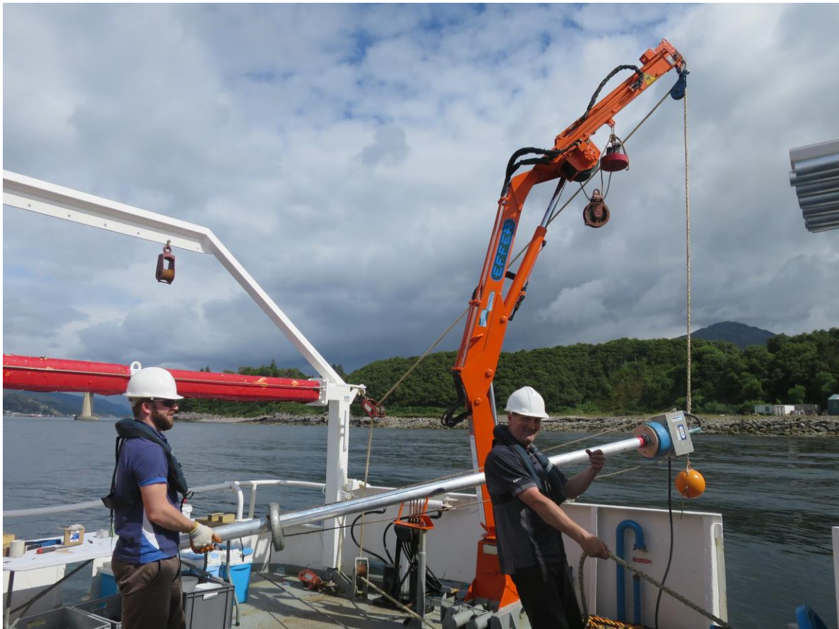
FIGURE 3 - SDI D-4 VIBROCORER ON DECK
