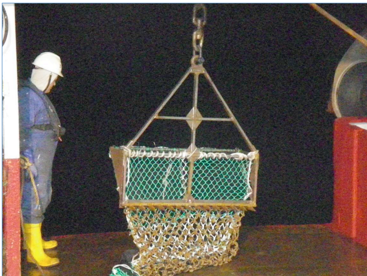
Figure 5.2 Modified 1.24m Shellfish Dredge Used
