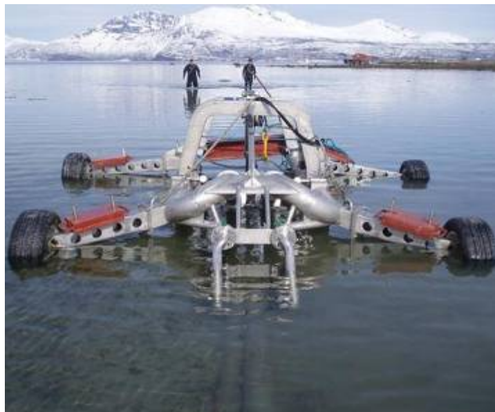
Figure 8.3 DPT5 high pressure shallow water jetting system
