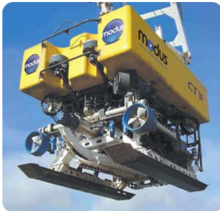
Figure 8.2 Typical Jetting Trencher
