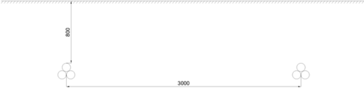
Figure 6.2: Two HVAC circuits with trefoil layout
