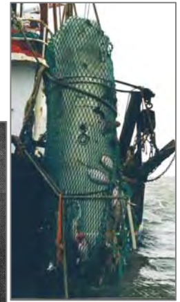
GC mine caught in fishing gear. Note the parachute housing still intact
