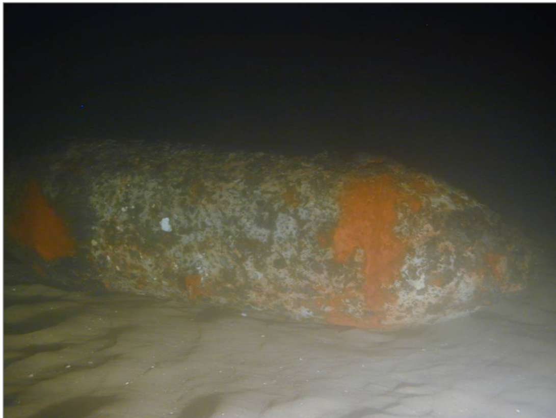
1000lb British high explosive bomb recovered by BACTEC in the North Sea in 2006
