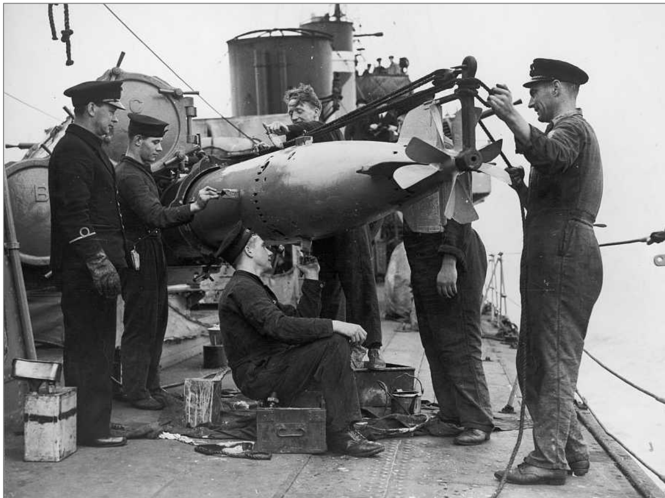
Preparing a torpedo aboard HMS Vanoc in August 1941 This is probably a Mark II or Mark IV torpedo
