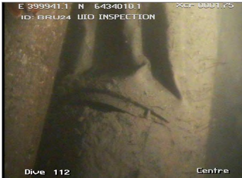
View of front of torpedo showing collapse of outer case and partial separation of warhead from pressure vessel
