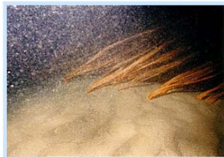
RE-INFORCED SEDIMENT BANK NEAR FULL DEVELOPMENT WITH A FEW SHORT LENGTHS OF FRONDS EXPOSED
