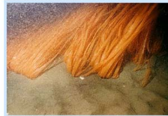
CONTINUED SEDIMENT BUILD-UP IN CENTRE OF THE MAT AND SLOPING TO AND BEYOND THE MAT EDGES.
