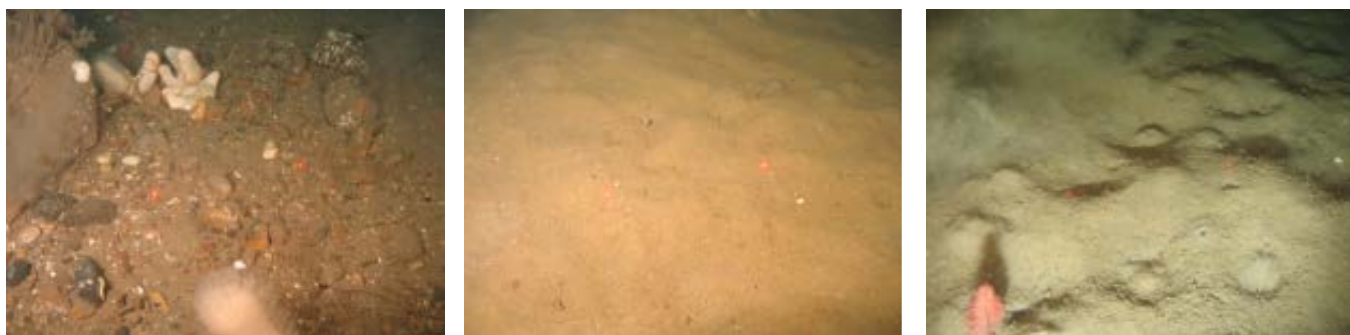
Figure 8.8: Representative seabed sediment photographs. (Left) – Sandy gravel and boulders from areas of Wee Bankie, sample no. 35; (Middle) - fine to very fine sand, sample no. 33; and (Right) - Muddy sand, sample no. 31. Note: the difference between fine/very fine sand and muddy sand is difficult to distinguish visually. Source: Appendix 14.1: Benthic Ecological Characterisation Survey
