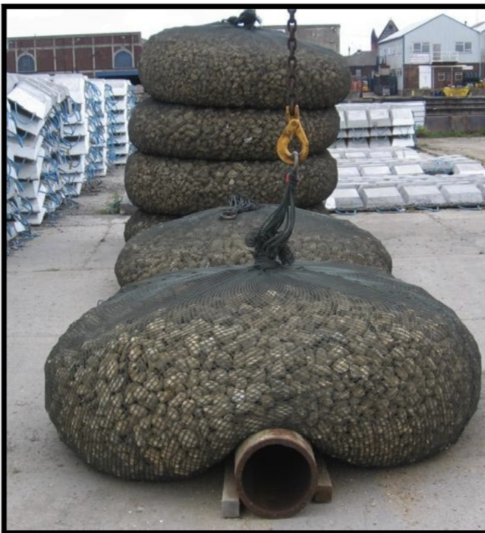
Figure 9: Rock Bag Cable Protection
