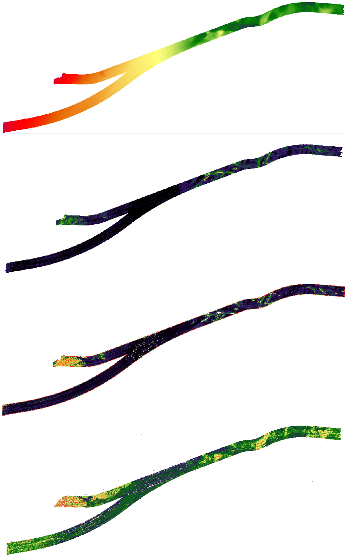
Figure 4: Images used in the integrated analysis for the ECR: From top to bottom: - Bathymetry; Slope; depth variability; Side scan backscatter
