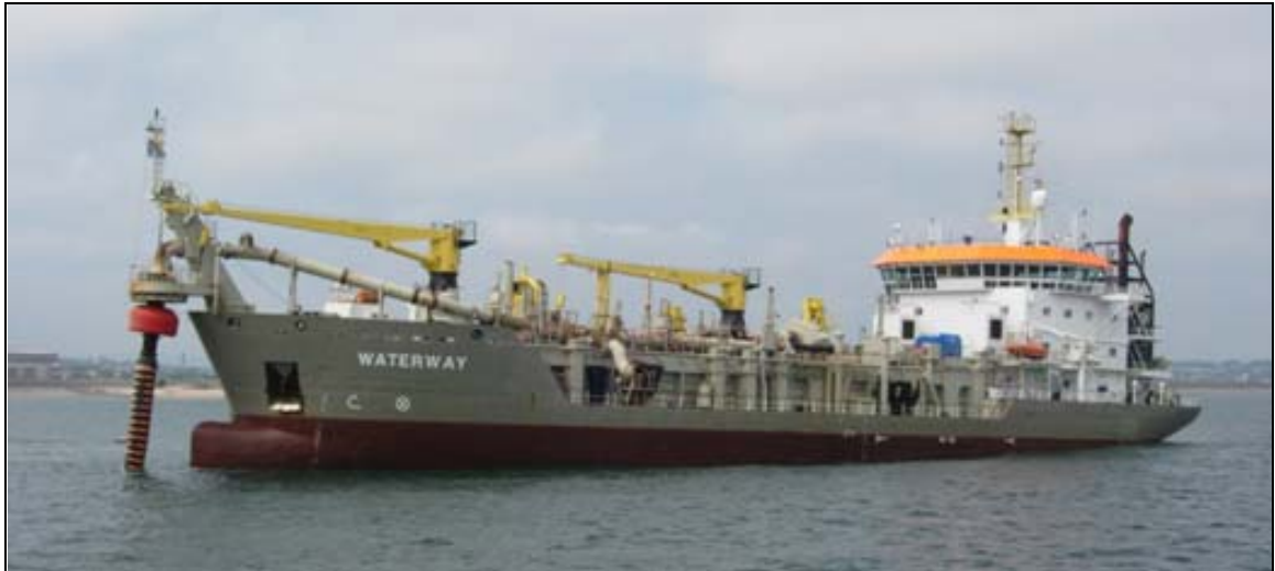
Plate 2.1 Example TSHD discharging via a pipeline from the bow
