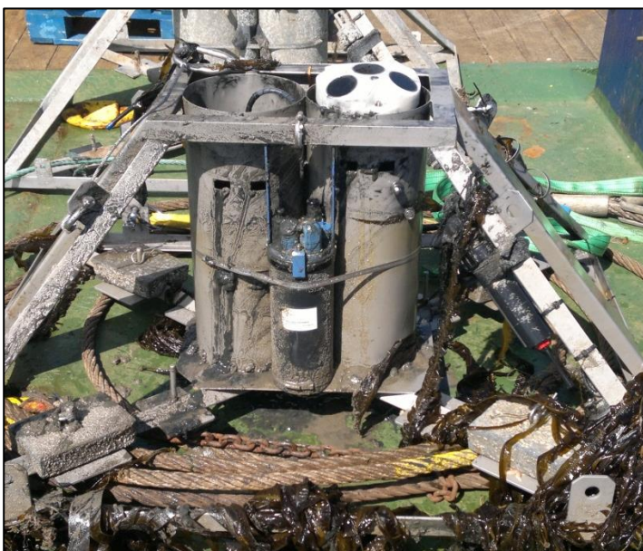
Plate 3.2 West Seabed Frame on Recovery Showing Sediment Covering Seaguard Sensors
