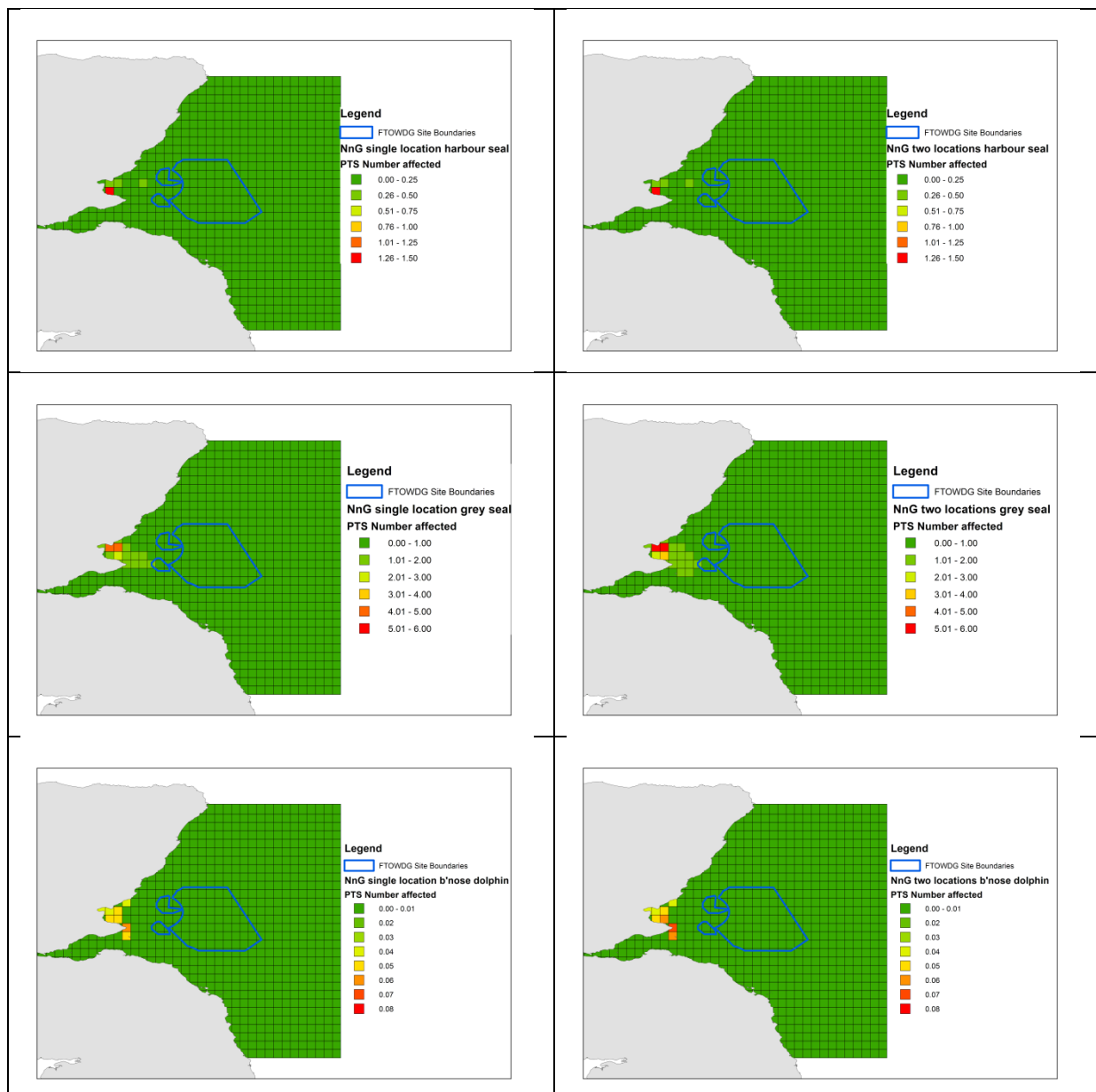
Figure 6. The number of animals predicted to experience PTS per 0.083 deg grid cell within the area of calculation (boundary of green area) for Scenario 1, single location (left hand panels) and Scenario 2, piling at two locations simultaneously (right hand panels), for both harbour seals (top panels) and grey seals (middle panels) and bottlenose dolphins (bottom panels). Note that the scale differs between species.
