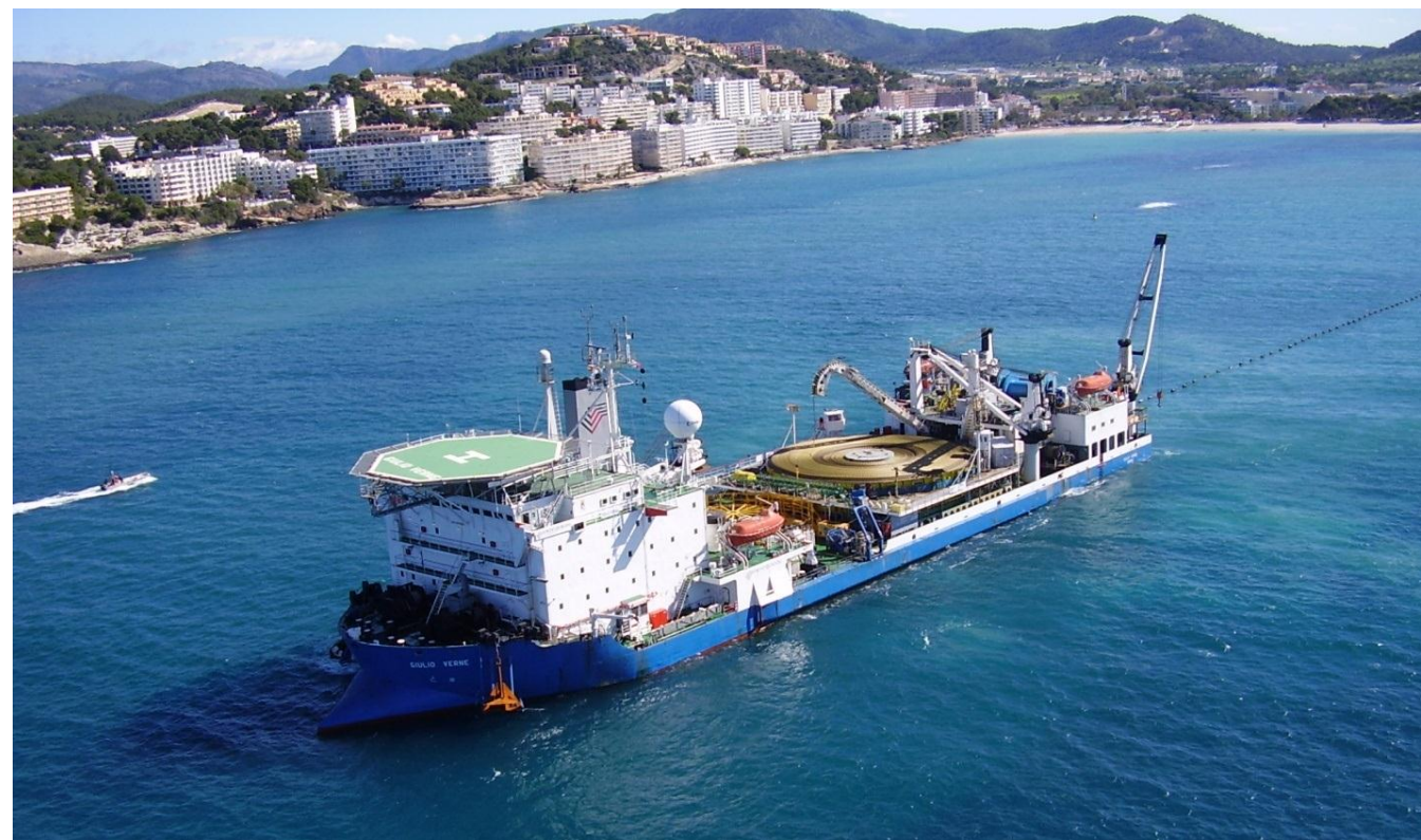
Figure 5.30: Cable lay vessel Giulio Verne (Source: Prysmian Group)
