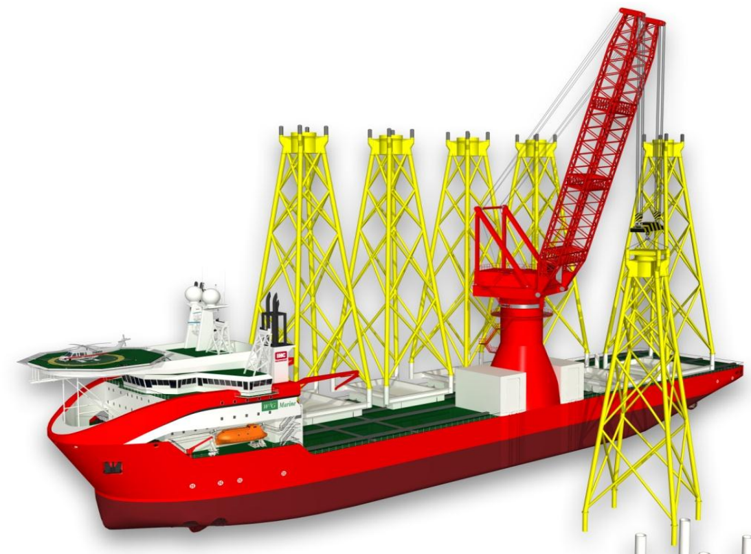
Figure 5.15: Transportation and installation vessel concept (Source: W3G Marine 2012)
