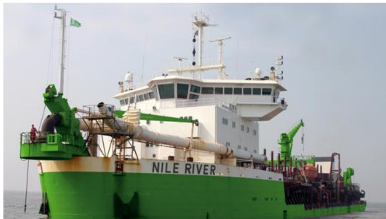
Figure 5.8: Dredging vessel – suction dredger (Source: DEME Group)
