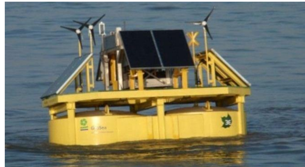
Figure 5.3: Typical floating LiDAR structure with mounted meteorological recording instruments (Source: Subsea World News 2011)
