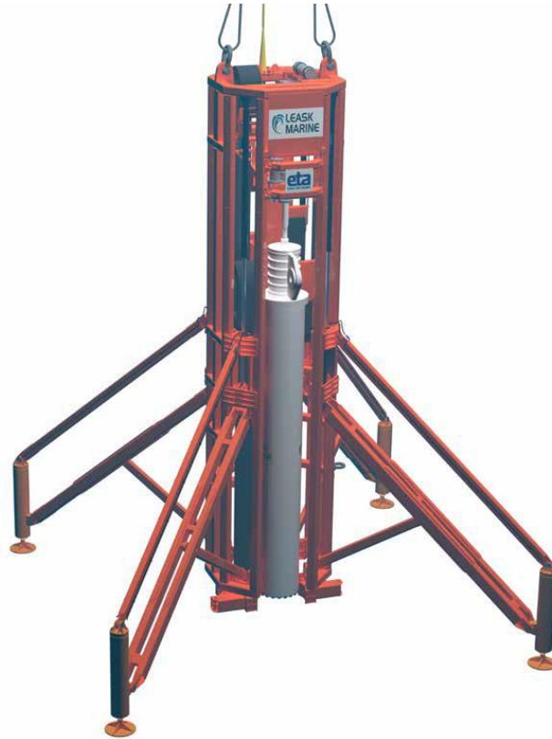
Figure 1. Leask Marine Submersible Drilling Rig (SDR)
