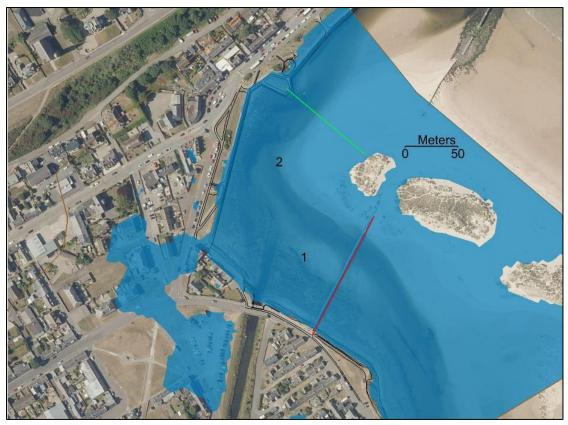
Figure 2.4: Water level at 200 year + climate change fluvial flood in Lossie combined with HAT adjusted for climate change
