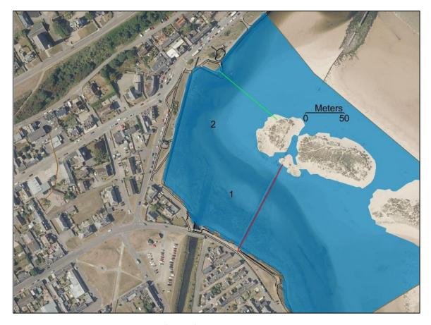
Figure 2.3: Water level at 200 year fluvial flood in Lossie combined with HAT
