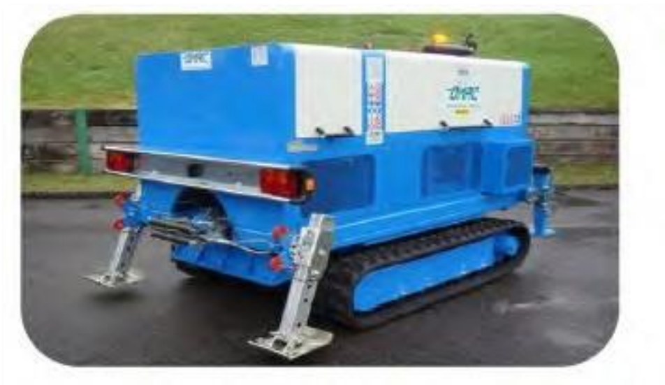
Figure 10: Tracked 10Te Bull Wheel Winch
