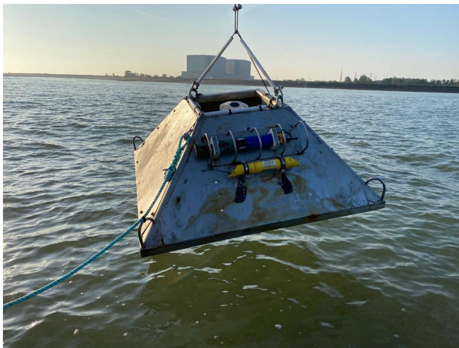
Figure 4: Example of ADCP deployed inside protection frame
