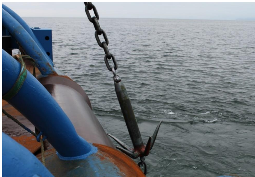
Figure 4-6 Grapnels and Chain at Stern Roller of Vessel
