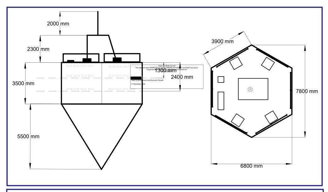
KAMES FISH FARMING LIMITED FAST FIONA 100T CAPACITY FEED BARGE 1:100 @ A4
