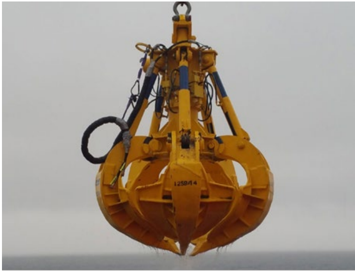
Figure 5-12 Example of boulder grab
