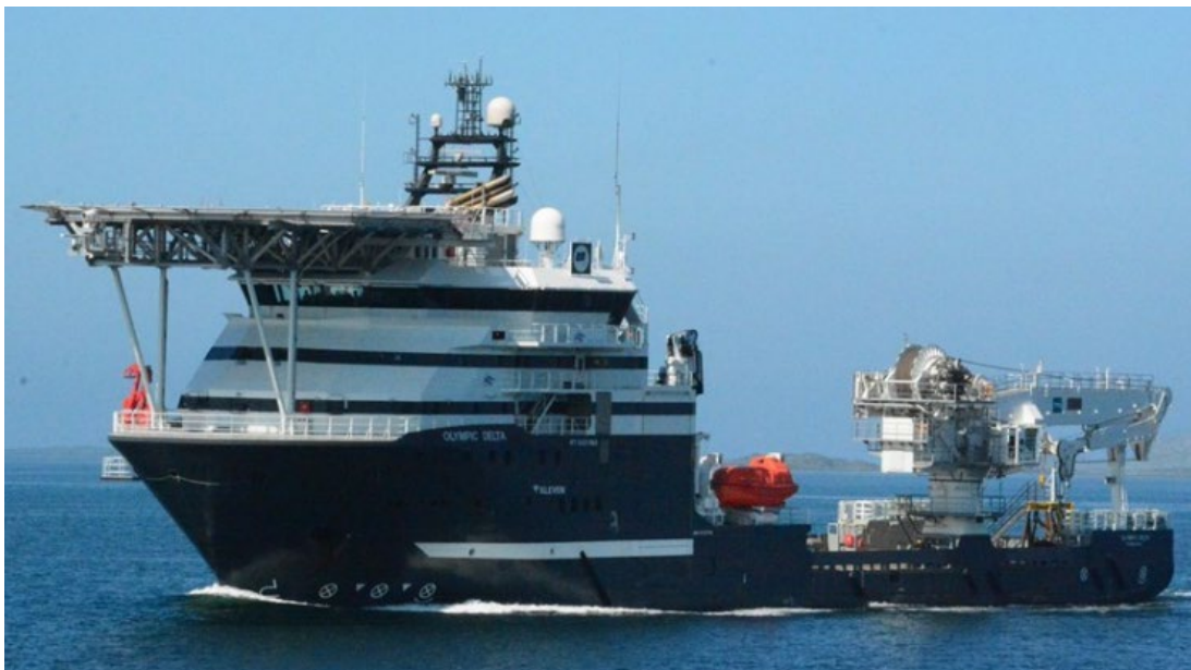
Figure 5-13 An example vessel used for boulder removal, crossing and stabilisation operations (DSS Olympic Delta)
