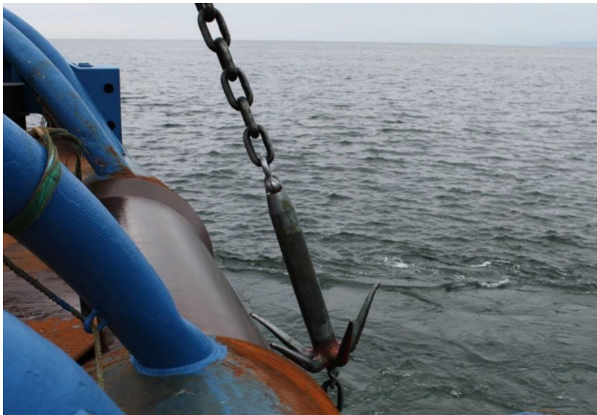
Figure 5-15 Example of grapnel and chain at stern roller of vessel
