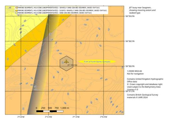
Site map overlaid onto BGS seabed sediment data.
