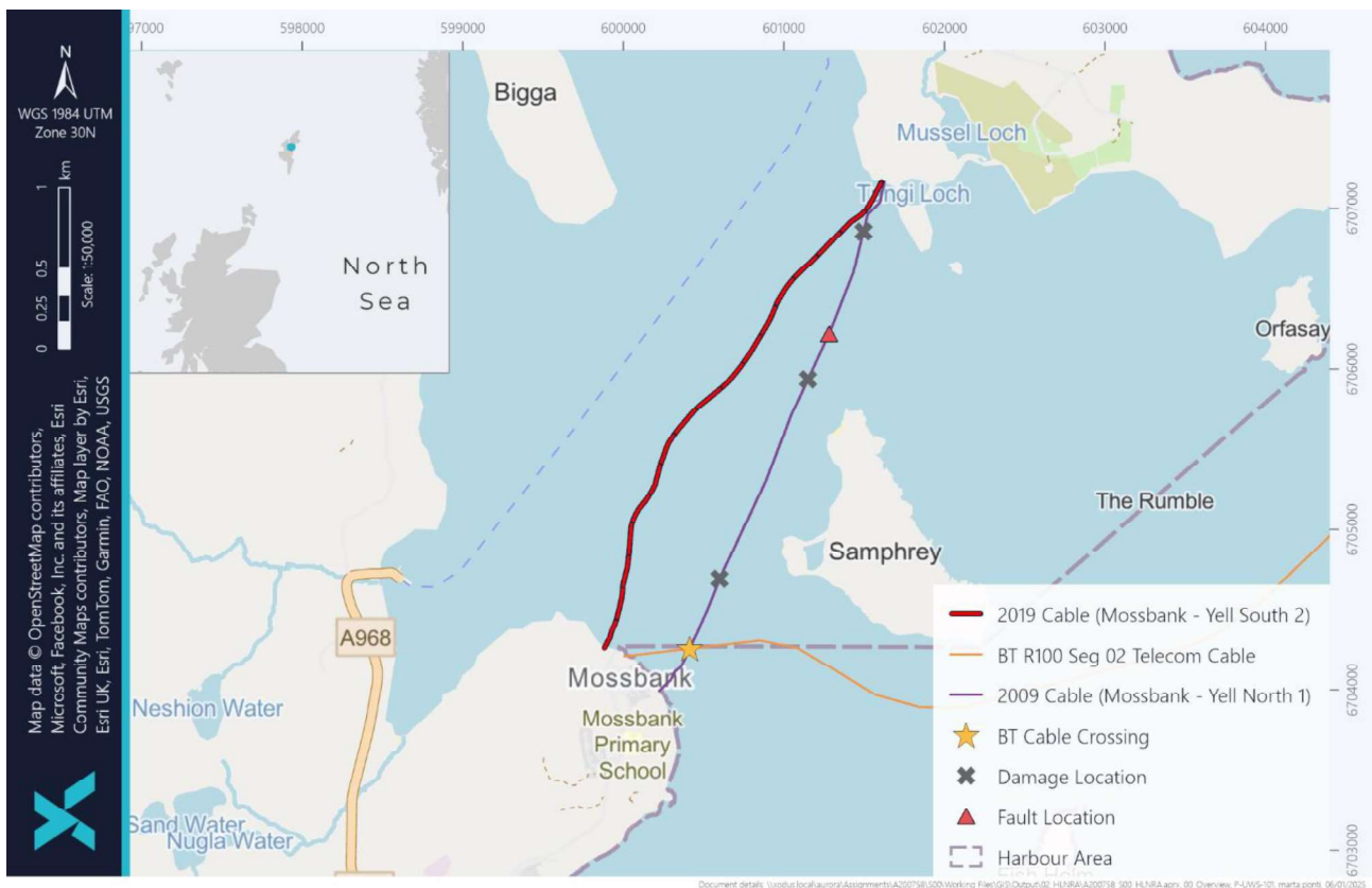
Figure 1-1 Existing subsea cable locations and fault and damage locations
